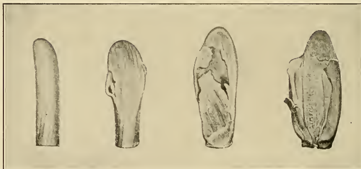
Fig. 873.—Four common types of lateral Mauser ricochet bullets (from Makins' "Surgical Experiences," etc.).
